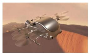
and the early Earth before life began. It is equipped with 8 rotors and the rotorcraft operates similarly to a large drone. It will be powered by a radioisotope power system. It will spend most of its time on the moon's surface making science measurements.
