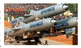
**cruise missile** in operation, capable of reaching speeds of **Mach 2.8 to Mach 3**. BrahMos can hit a target up to a range of 290 kms and can be launched from submarines, ships, aircraft, or land platforms. It has a **solid propellant booster engine**. It has a **very low radar signature**, making it stealthy, and can achieve a variety of trajectories.
